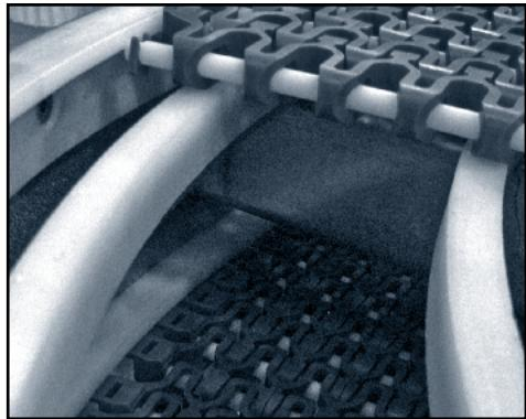
The hold-down profiles must not be in contact with the belt (see the pictures below):
