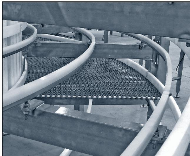
To make the fastening and the support of the belt, EUROBELT has designed two types of hold-down profiles with different geometries, but with the same uses and services.
