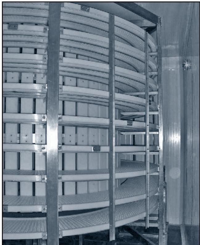
SERIES E93 can also be used for applications in spiral conveying systems. Its design of flat and rounded edges reduces considerably frictions between the inner curved radius and the drum, getting a smooth power transference from the central drum to the belt, having as a result a saving in energy costs.
