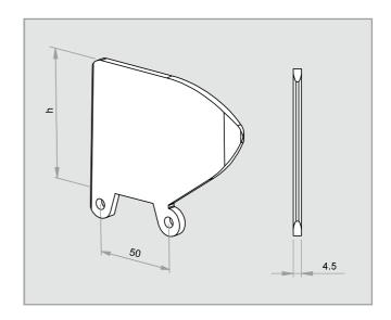
The **side guards** are plastic accessories to be inserted into the belt structure to retain the product laterally, avoiding overflows and frictions with the conveyor structure itself.
