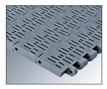
Eurobelt Series E50 Perforated Flat Top has an 18% open area, a completely smooth surface, and grille-shaped small straight holes without structural obstacles, to make easy the drainage of any liquid.
