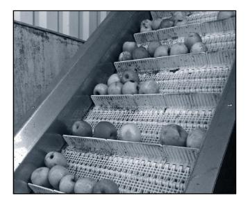
When building a conveyor, Eurobelt can design your belt with flights and/or side guards, taking into account the size and the weight of the product to be transported, as well as the height and inclination of the conveyor.
