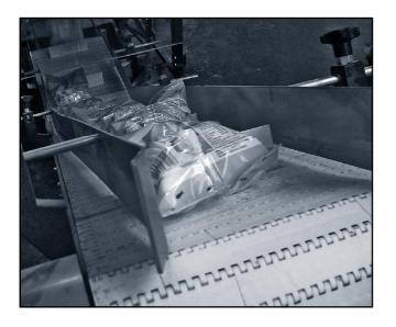
The **flights** are plastic accessories to be inserted across the belt. They are used to push the product in ascent, descent or accompaniment applications, avoiding that it slips along the belt.
