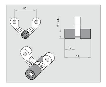
The distance between the side edge of the belt and the centre of the hold-down roller (indent) must be a multiple of 10 mm. Hold-down rollers cannot be used with the following sprockets:
