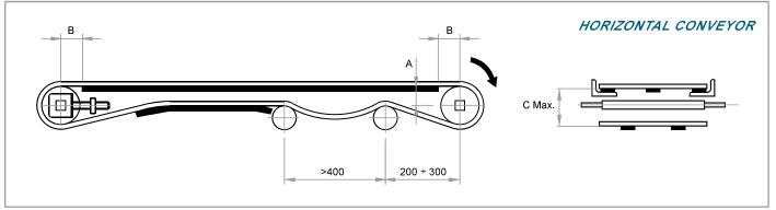
[A] Distance between the sliding surface of the belt and the centre of the shaft.
