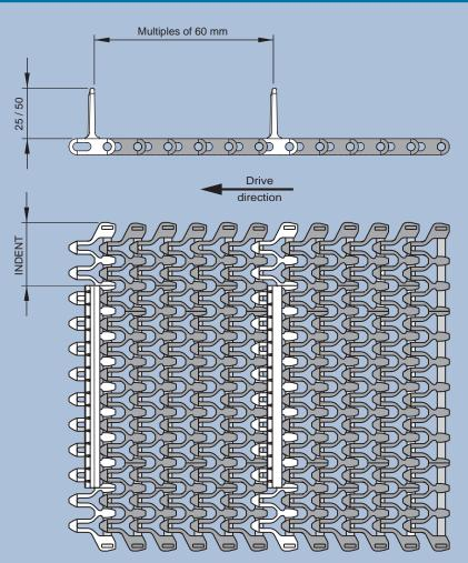
The E93 curve Series has no cling fights as an accessory for building elevating conveyors.
