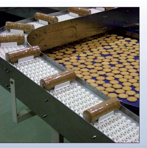
These flights give response to problems arising in elevating, descending and accompaniment applications, preventing the product from sliding on the belt.
