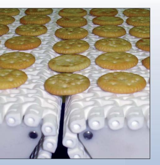
With a 12 mm pitch you will be able to carry out product transfers at high speed in minimum turn diameters.
